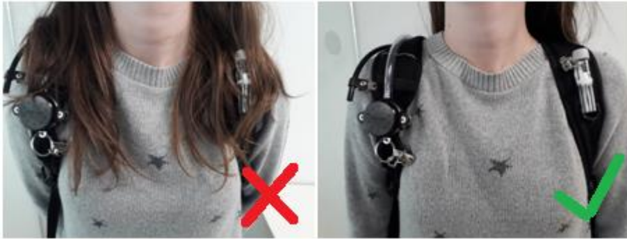
Figure 7. Correct placement of the NO 2 tubes on the backpack.
